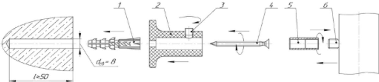
Attach the plastic part of the bracket 2 to the wall. Fasten with screw 4. Screw the nozzle 5 to the fixing screw 6 of the dryer until it stops. Follow these steps for all fasteners. Insert the nozzles 5 screwed to the dryer into the holes of the plastic fasteners 2 screwed to the wall. Fasten the attachments 5 with the screws 3. Before using it for the first time, wipe the dryer with a dry cloth and leave it at room temperature for at least 6 hours.
