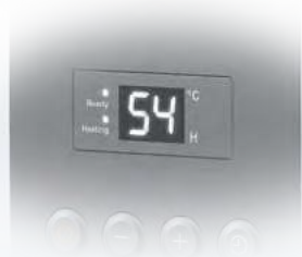
Indicator lights on and heating on the display
